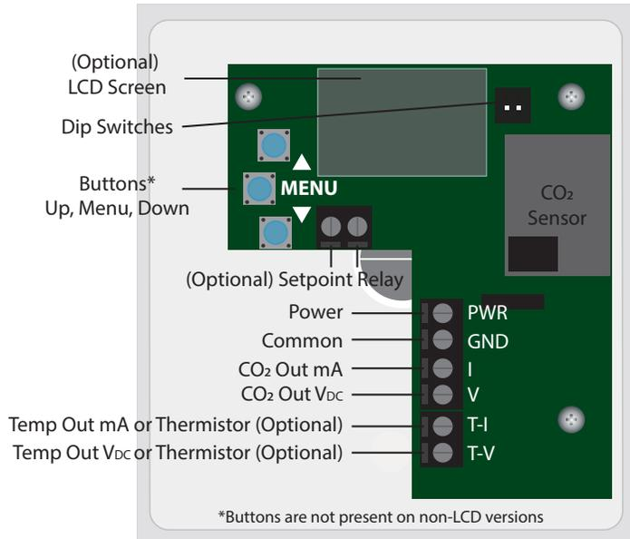
4. Set DIP switch positions to accommodate your application. DIP switch 2 only applies to units with transmitter temperature output selected.
